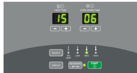
This economy control allows for the operator to select the ideal temperature, heating time and cooling time for each use.
