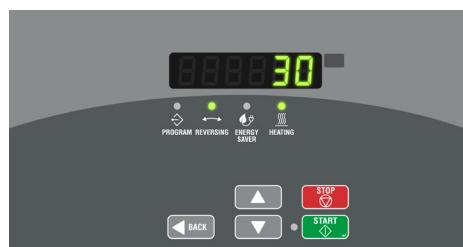
Our programmable control allows any combination of up to 30 auto-dry and time-dry cycles to be saved, providing easy user interface.
