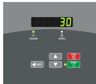
The M Series Control is designed to manage the drying and cooling cycles of the gear cabinet. The controller is programmed to meet NFPA standards with the flexibility for the operator to adjust the time settings.
