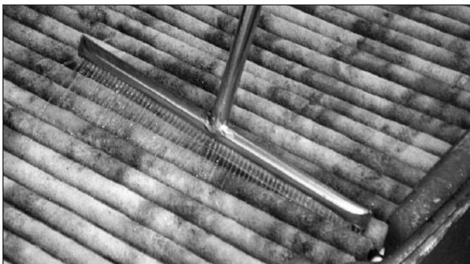
If you need to clean the sheets, remove the RSV so that solids can freely drain back to the tank. Then clean the sheets one by one with the
