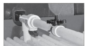
not, remove them at this time. Verify that the lateral inlet valves in the pods are open and the spray nozzle turbines are pointed up, as shown below.
