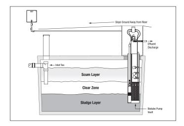
Vaults should be examined to determine if cleaning of the Biotube filter is necessary. If the liquid level inside the vault is discernibly different from the level outside the pump vault while the pump is running, cleaning is required. Remove the filter cartridge and clean it following the applicable instructions in Appendix B.
