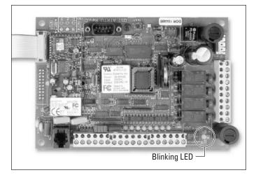
On MVP, Simplex, and Duplex panels, turn on the control circuit, then toggle the pump "AUTO-OFF-MAN" switch to "MAN." The motor contactor will visibly and audibly engage at this point. If the motor contactor does not engage and there are no alarm conditions, refer to the wiring diagram and verify the connections on the control circuit were properly terminated.
