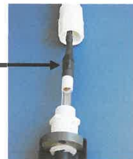
Apply Dielectric Grease to the inside of the boot. Lamp Cord Connected and Lamp Inserted into the Aluminum Frame.
