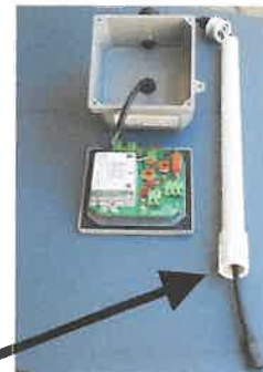
Threaded Bottom End of PVC Handle
