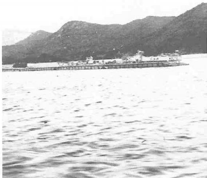
Pontoon causeways played an important part in many of our landings. Above is a causeway awaiting a "marriage" with an LST.
