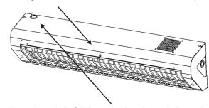
12. Turn the unit switch ON by pressing the switch on the top left corner.
