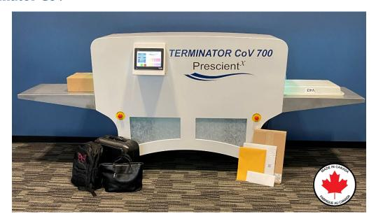
The Terminator CoV is a transportable continuous high volume UVC disinfecting conveyor system.
