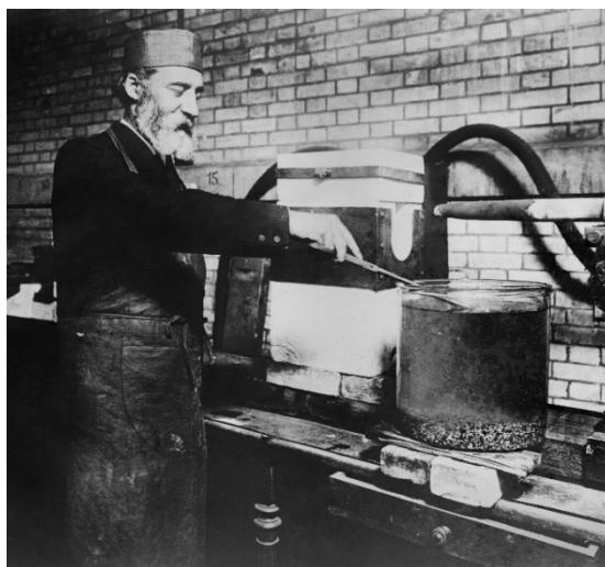
Henri Moissan quenching cast iron (next to the arc furnace he invented). 9
