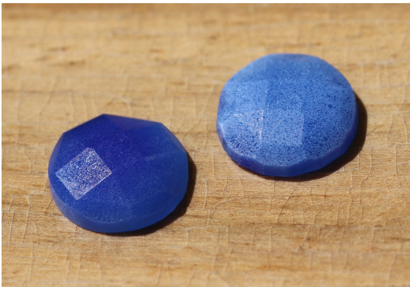
Two galaliths, produced by the author using the dry method and faceted by Eric & Janet Mitchell. Each stone has a diameter of 8mm.
