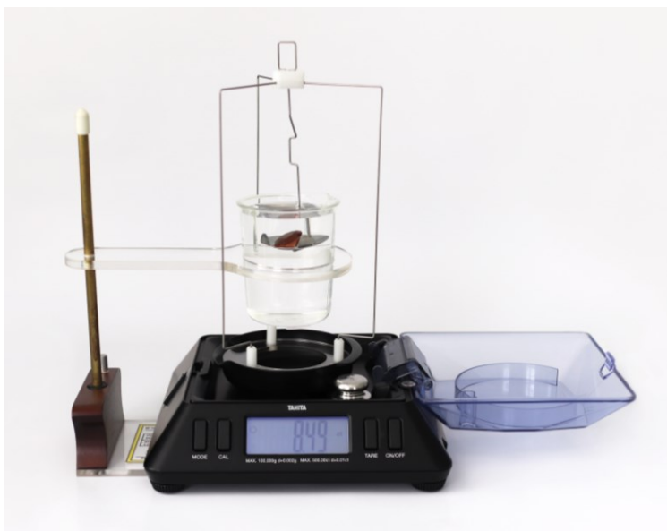
Measuring specific gravity with a Tanita KP-601 scale and a specific gravity kit from Mineralab.
