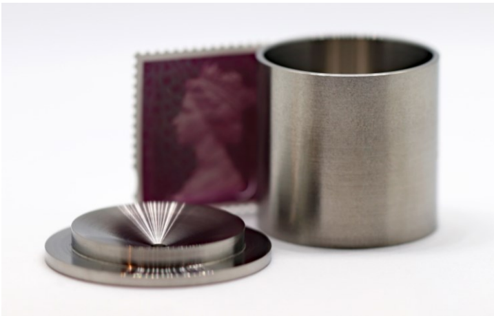
A pycnometer, manufactured by GARDCO and sold by Lustre Gemmology (postage stamp for scale).
