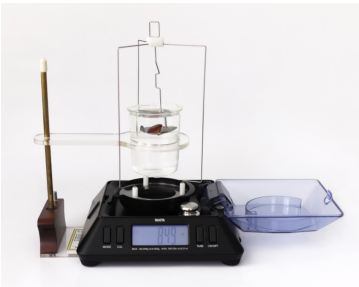
Measuring specific gravity with a Tanita KP-601 scale and a specific gravity kit from Mineralab.
