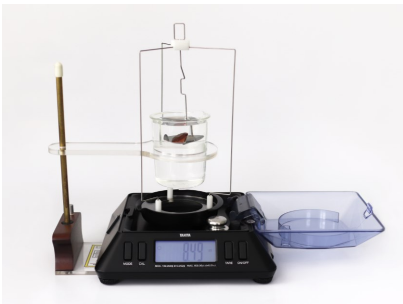
Measuring specific gravity with a Tanita KP-601 scale and a specific gravity kit from Mineralab.
