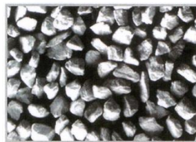
Cast Tungsten Carbide+Ni Alloy Matrix
