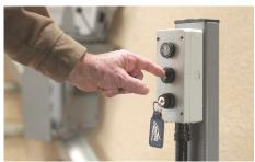
Landing controls allow the stairlift to be called or sent. A keyswitch can completely immobilize the stairlift to prevent unauthorized use.
