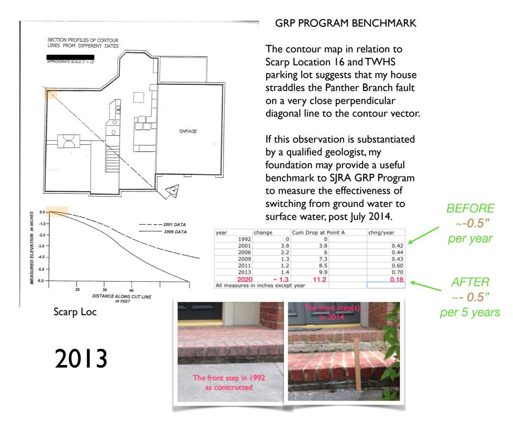
Subsidence at fault line before and after the GRP pipeline became operational in 2015
