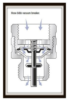
With loss of water supply pressure, disk seals against diaphragm, checking backflow and opening vent ports.
