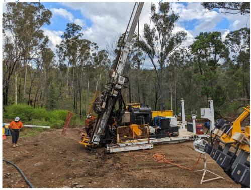
Pictured above, the diamond drilling rig restarting the hole below Goldsmith's Reef targeting a geophysical bullseye anomaly at circa 250m depth.
