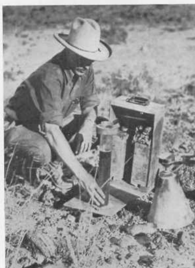
Dr. Forrest Shreve reading an instrument which records changes in circumference of cacti trunks to which it is attached. Daily and seasonal variations are due to changes in water-balance.
