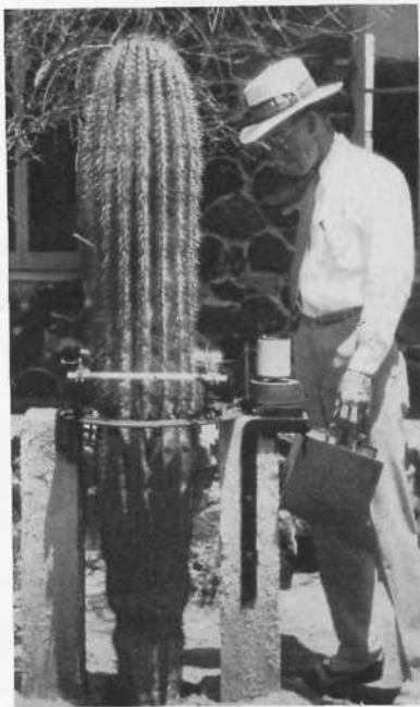
Dr. T. D. Mallery reading the long-period rain guages. Light oil is used in the guages to prevent evaporation of captured rain-water.
