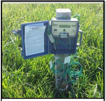
**Figure 2.** Automated Soil Moisture Recording Device for Watermark<sup>TM</sup> Sensors.
