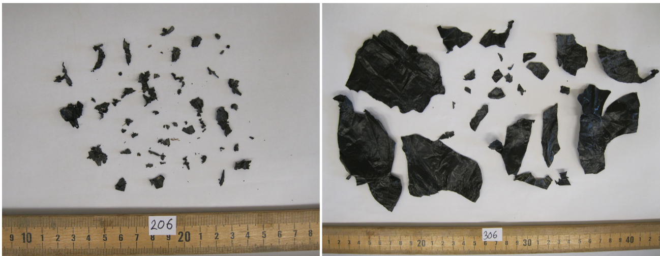
Figure 3. Samples of plastic BDM Naturecycle, approx. 20% biobased ( left ), and an experimental polylactic acid (PLA)/polyhydroxyalkanoates (PHA) mulch, 86% biobased ( right ), recovered six months after soil incorporation in the field at Mount Vernon, WA (ruler units are cm). (Photos by S. Ghimire)
