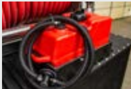
3 gal fuel tank with copoly mounting bracket
