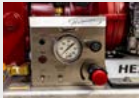
Completely enclosed control panel with on/off start, low pressure protection override, vernier throttle, choke, liquid filled gauge, low oil light, & light shield with LED light
