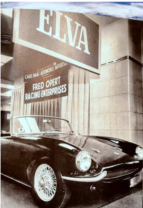
Left: Connie Schuchard's Courier Mk IV 'T' Type, Ford Cortina 1500 powered, four wheel discs, and new 'Tru-Track' suspension, built for the London Earls Court Auto Show. Right: One of two Courier Mk IVs owned by Fred Schuchard, also 'Tru-Track' but MGB 1800 powered.
