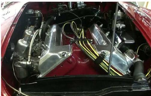
The temperamental engine was notorious for warranty problems during the course of production, and sales dropped quickly. The engine suffered from detonation and burnt oil. Most of the problems with the Twin-Cam engine were rectified with the low-compression version, but by then the damage had been done. The Twin-Cam was dropped in 1960 after 2,111 (2,210 according to some) had been produced. Production ended in April 1960, but had slowed to a trickle long before.
