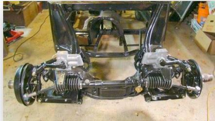
Next was restoration of front and rear suspension. Cleaning, painting and replacing all bushings and seals. I also replaced the entire brake system with new master and brake cylinders and brake lines. The Differential was inspected and cleaned. In good condition. No repairs needed.
