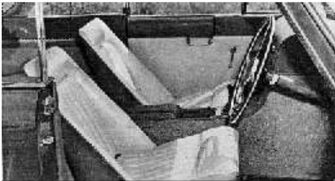
*On a column 4in. shorter than a standard is a steering wheel of black and red plastic laminations. Instruments are normal M.G. fittings but the control knobs are sensibly varied in shape.*
