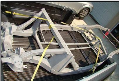
Luckily, the frame was in pretty good shape. It had a few holes and spots of rust, but after sand blasting, I only had a few spots that needed to be fortified with metal and other welded patches.
