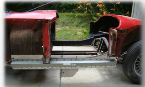
The sill and other body panel replacement project took me most of Spring 2008 through June of 2009. I was also still sanding paint off of everything. In July of 2009, after welding in a couple of bracing pipes to the top of the cockpit to keep the body from folding in half, I removed the body from the frame.
