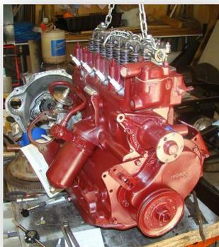
I finished up the Trans in February 2010 and took the engine block to my machinist friend Alan Olsen, who re-bored and honed the cylinders to .060. Added new Rings, Valves, Tappets, Push Rods and Guides. The Head was also honed and polished and a new Timing Chain installed. Put it all back together with new gaskets and painted it MG red.
