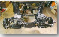
Next was restoration of front and rear suspension. Cleaning, painting and replacing all bushings and seals. I also replaced the entire brake system with new master and brake cylinders and brake lines. The Differential was inspected and cleaned. In good condition. No repairs needed.
