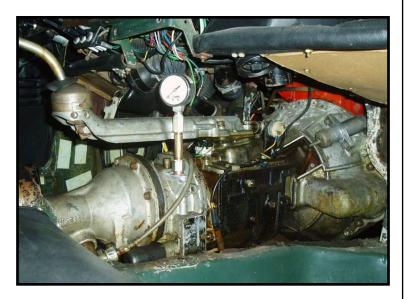
hit the overdrive switch. Of course, nooooo pressure. Was not surprised. After the test I decided to consult with my cousin Dave Faulls, an ex-mechanic and a retired mechanics teacher. After explaining the problem and looking at the overdrive diagram in the service manual, he said it sounded like a part could be missing. I thanked him for the advice and shortly after I removed the main components from the chassis I decided to take a break from the chassis clean-up work on the
