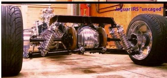
It is well known that when a differential assembly is bolted to the chassis, there is a great amplification of gear noise. There must be rubber insulation of some kind, and lots of it. In addition, on any frameless type of body, we have the problem of finding attachment points for the rear suspension which will be strong enough. This last is a special problem with I.R.S. where the pivot points often come in very awkward areas: places where
