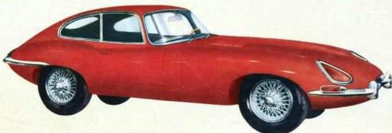
the automotive press about the Jaguar XK-E. 150 mph maximum speed; 265 bhp at 5500 rpm; disc brakes and independent four-wheel suspension; lightweight, aerodynamic stressed
