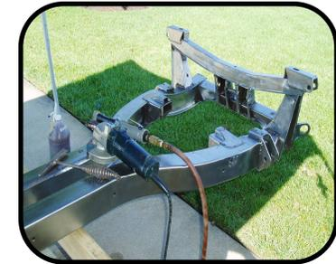
To seal the holes I used duct tape, not perfect but much better than masking tape. Once the holes were sealed I first poured in about a gallon of Purple Power de-greaser, rolled the chassis several times, drained it and gave it a good rinse with hot tap water. Drained out the water the best I could, than let it sit for several days in the sun, and also rolling it during the drying period.
