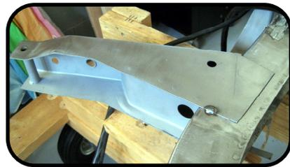
As most of us well know, when removing and replacing any part of a chassis the alignment of the new part is very critical. I found that a measuring tape, straight edge and square is not enough. In my case, I set the outriggers in place, then lowered the body in place, installed all the bolts then tacked the outriggers in place. It takes time but it's a guaranteed fit at the end. Once the repairs were complete I moved on to the next job. Are you all ready?
