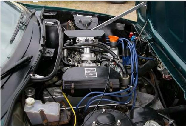
The car's smooth and flexible 3.5-liter aluminum V8, which was a descendent of the engine GM introduced in its 1961 Buick Special, Olds F85 and Pontiac Tempest, weighed little more than a cast-iron four. With federally mandated smog equipment (including twin catalytic converters), the twin-carbed Zenith-Stromberg version put out 133 horsepower and 174 lb.-ft. of torque; the Lucas-injected California version put out 137 horsepower along with 168 lb.-ft. of torque.
