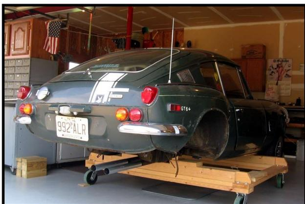
The first sections of the car that I decided to tackle were the differential and rear suspension. Raised the car up on jack stands and commenced the disassembly. Suspension first and then the differential. After this step I decided that I would need some type of a large dolly to put the car on for maneuverability.
