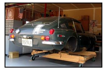
The first sections of the car that I decided to tackle were the differential and rear suspension. Raised the car up on jack stands and commenced the disassembly. Suspension first and than the differential. After this step I decided that I would need some type of a large dolly to put the car on for maneuverability.
