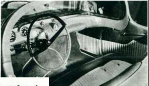
Windshield frame, with laminated steel roll bar, takes stock GM truck glass and fittings. Inverted, the unit curves over the cockpit, protecting the passengers from wind.
