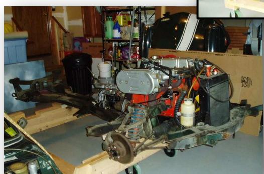
*Keep in mind, that before removing the bonnet, body, engine and drive train I had to unplug and label all electrical wires, disconnect and drain hydraulics lines, and detach all cables and linkages.*
