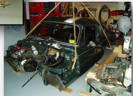
One thing I forgot to do was to completely drain the brake master cylinder. Even though only a minute amount of brake fluid remained in the cylinder it was enough to damage it beyond repair. The clutch master cylinder and slave cylinder seem okay.
