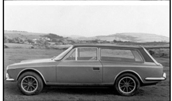
The first Estate also had redesigned rear damper mountings. The Invader saloon body shell is distinguished from the Genie by different (smaller) rear lights and side vents were added to the rear roof pillars. The bonnet vents were also changed from front to rear-facing, albeit that some were fitted with the Genie type.
