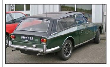
All exterior door handles were flush. Mk Is and most Mk IIs have Gilbern-unique flush rectangular chrome door handles with hidden latch releases, but some later Mk IIs were fitted with the Triumph Stag type, as are nearly all Mk IIIs. Other features, such as opening front quarter lights and rear side windows, may be present on some Mk Is but these were all fixed on Mk IIs.
