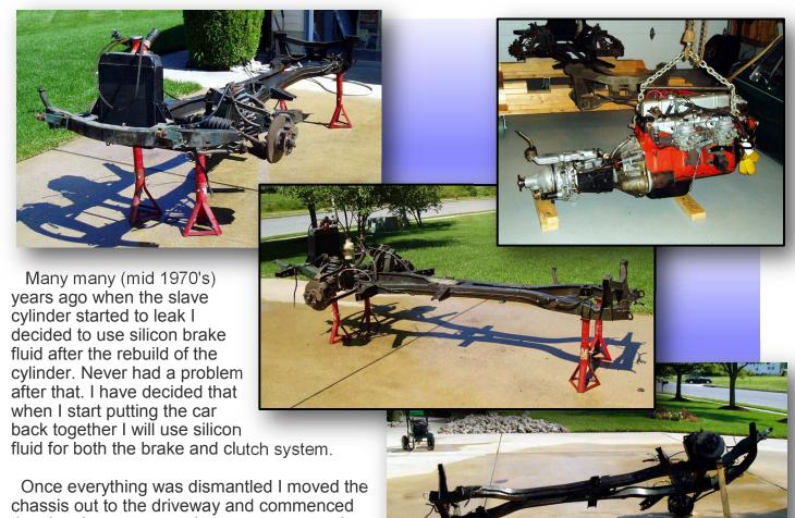
Once everything was dismantled I moved the chassis out to the driveway and commenced the cleaning process using a pressure washer. This got rid of most of the loose dirt. To remove the oil residue I needed to use
