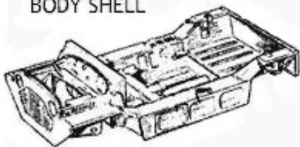
The Moke's construction is simple. The body mainly consists of two box-section "pontoons" or "side boxes" running between the front and rear wheels, and include (non-hollow) extensions of that from the back of the car all the way up to the front. These are connected by the floor pan, the firewall and a sturdy lateral torque box that runs under the
