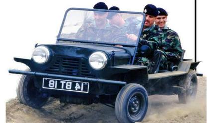
In a further attempt to make something for the army, a few four-wheel drive Mokes were made by the addition of a second engine and transmission at the back of the vehicle with linked clutches and gear shifters. This did nothing for the ground-clearance problems, and mechanical complications discouraged development beyond the prototype stage. This vehicle was called "The Twini" and was shown to the US Army—again with no success.
