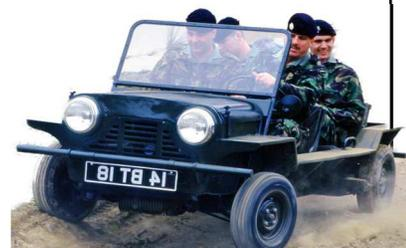
In a further attempt to make something for the army, a few four-wheel drive Mokes were made by the addition of a second engine and transmission at the back of the vehicle with linked clutches and gear shifters. This did nothing for the ground-clearance problems, and mechanical complications discouraged development beyond the prototype stage. This vehicle was called "The Twini" and was shown to the US Army—again with no success.
