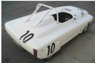
Mechanical is all stock, Moke chassis, driving position had moved to far back, high quality fiber glass body. Lowered and modified suspension. Pax shocks and Panasport competition wheels. As you might expect considering its racing origins, the interior is pretty sparce. You can see the Moke dash, pedals, and interior panels clearly.
