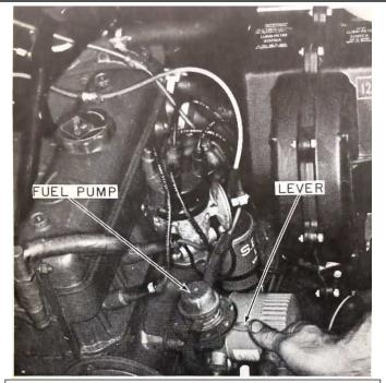
Some fuel pumps have levers to prime the carburetor in the event that you run out of fuel. The lever can also be used to test the fuel pump.
