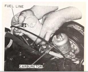
Testing the fuel pump output ( test 1 )
