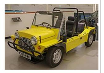
vas plant. Initially these Mokes were identical to late-model Australian Mokes; very soon, however, they were altered to use then-current British production Mini saloon components, including the standard-length Mini rear trailing arms and the 12–in wheels with modern low-profile tires, which the saloon had acquired during the Moke's absence from Europe.
