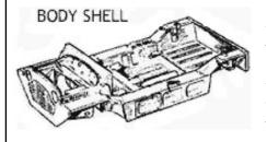
The Moke's construction is simple. The body mainly consists of two box-section "pontoons" or "side boxes" running between the
