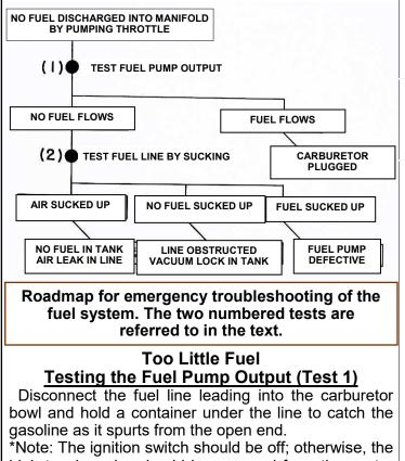
high tension wire should be removed from the center of the distributor cap to prevent the possibility of the engine starting and spraying gasoline all over the engine compartment !! If a good size stream of fuel flows from the pipe, and the trouble has been isolated to the fuel system, the defect must be in the carburetor. If no fuel flows, the trouble must be in the pump, lines, or gas tank.
