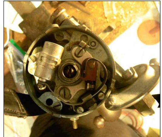
*Notice the condenser bracket interfering with the distributor cam.*
