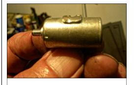
There's a groove worn in the condenser bracket by the distributor cam.
