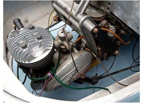
Reverse gear of a sort was offered on later models, but using this involved stopping the engine and starting it backwards. This was done by reversing the Dynastart unit, a device which doubled as both starter and generator. It operated as a starter motor when the starter button was pressed but when the engine was running it generated power instead and recharged the battery.
