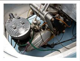
using this involved stopping the engine and starting it backwards. This was done by reversing the Dynastart unit, a device which doubled as both starter and generator. It operated as a starter motor when the starter button was pressed but when the engine was running it generated power instead and recharged the battery.
