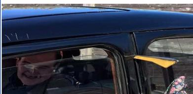
Trafficator. These are early British turn indicators. They are normally retracted into the doorpost and pop up—and flash—when activated to indicate a turn. It just shows how far ahead the Brits were considering it's been only in the past few years that modern car makers have installed indicators above the fender line.
