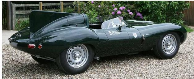
Innovative monocoque construction and aerodynamic efficiency integrated aviation technology in a sports racing car, some examples including a renowned vertical stabilizer. Engine displacement began at 3.4 litres, was enlarged to 3.8 L in 1957, and reduced to 3.0 L in 1958 when Le Mans rules limited engines for sports racing cars to that maximum. D-Types won Le Mans in 1955, 1956 and 1957.
