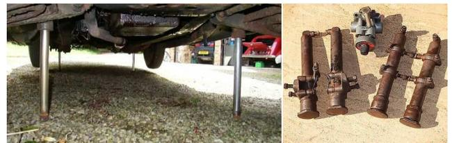
This is an example of the amazing Smith's Jackall System' which consisted of four hydraulically activated rams that were bolted to the chassis, two at the front and two at the rear. The jacks were connected to a Jackall Pump on the bulkhead that enabled the front, the back, or the entire car to be raised to facilitate a wheel change.
