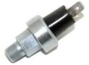
The TR6's oil pressure switch is crucial, he says. "It may look great to have the original switch under the hood, but this \$15 part triggers the idiot light, **and if someone doesn't notice the mechanical gauge, they will be in for a major engine rebuild or a new engine altogether.**"
