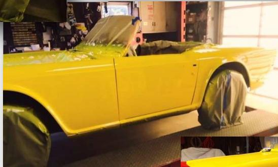
Wet sanded with 2000 grit paper and buffed out. Installed a new wiring harness after frying the first one because of a wire on the wrong terminal, new wood dash and interior from TRF as well as the convertible top.
