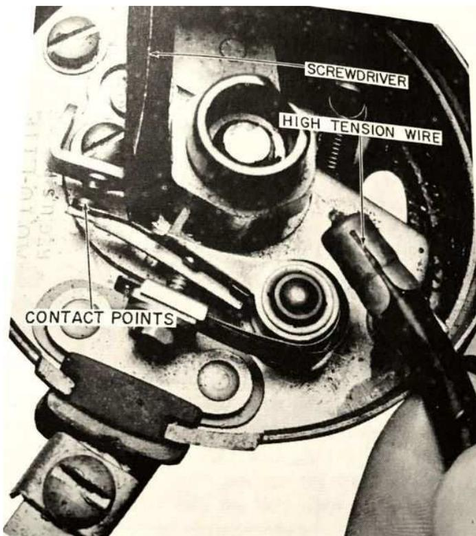
Opening and closing the ignition points with a screwdriver (TEST-1), while holding the main high tension wire close to the metallic part of the engine, is a simple test of the primary circuit
