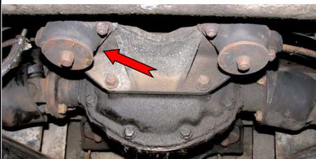
Other potential trouble areas seen in many TR6s include the front passenger side rear differential mount ( "This rubber mount is usually forgotten, and when it deteriorates, it causes a big clunk," Mark cautions ), the pick-up points on the lower front A-arms ("If they're
