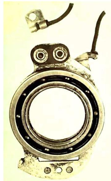
A broken primary lead may not show up until you pull on it. The insulation hides the damage.
