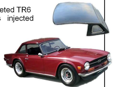
Although it was never subjected to a visage-altering bumper swap like the MGB, the TR6 received a few changes. Regulations required two stages of TR6 bumper alteration. For 1974, large black rubber overriders were fitted to the standard chrome bumpers front and rear, and for the car's last two years, the front bumper was raised to just below the headlamps, necessitating new turn signals set below the bumper.
