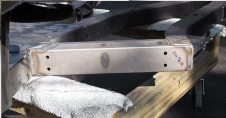
"You'll have to inspect the frame at the rear trailing arm assemblies--they didn't have any weep holes to allow moisture to get out. On the body, the floor pans and the rocker panels under the doors are trouble spots, as are the areas where the rear fenders and deck meet and the lower rear portion of the front fenders- the cowl vent drains into this fender area, and leaves can get in there and clog the drain hole," he explains.
