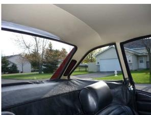
Factory hardtops are double-insulated which helps greatly increase the warmth compared to that soft top. The seals are good and can even make the car feel more strengthened and stiff. One thing that requires attention when installing the hardtop, is tightly fastening the six mounting bolts.
