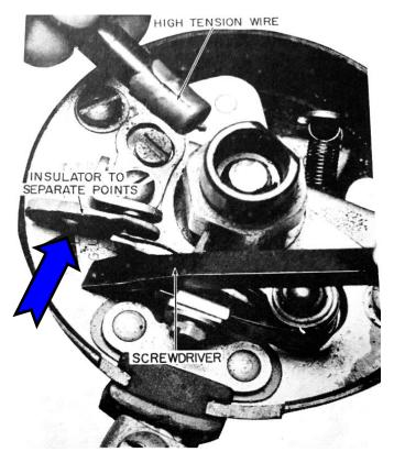
Using the screwdriver as a set of points (TEST-2).
