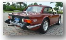
alteration. For 1974, large black rubber overriders were fitted to the standard chrome bumpers front and rear, and for the car's last two years, the front bumper was raised to just below the headlamps, necessitating new turn signals set below the bumper.
