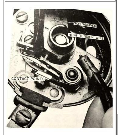
Opening and closing the ignition points with a screwdriver (TEST-1), while holding the main high tension wire close to the metallic part of the engine, is a simple test of the primary circuit
