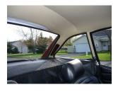
Factory hardtops are double-insulated which helps greatly increase the warmth compared to that soft top. The seals are good and can even make the car feel more strengthened and stiff. One thing that re-
