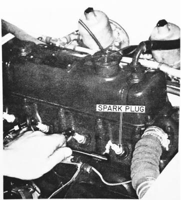
Testing the ignition system for a spark to the spark plug terminal.
