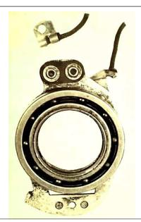
A broken primary lead may not show up until you pull on it. The insulation hides the damage.
