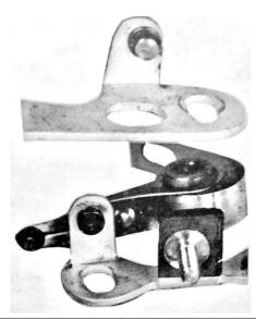
A sample of good ignition contact points (top), and a bad set (bottom) for comparison. A light gray contact surface is indicative of a set of contact points working at high efficiency. The lower set is burned black from either high voltage or oil.
