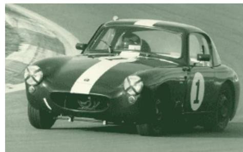
in un-sprung weight per wheel. Apart from alterations to the shock absorber valves and the addition of an anti-roll bar across the front, the suspensions remain exactly as per the production car.
