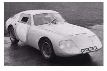
The body was developed from an original Healey idea, made as a mock-up and tested in the BMC wind tunnel before the actual final ver-
