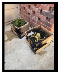
Per San Antonio Fire Department, the dry soil in the boxes caused a chemical reaction which caused them to spontaneously begin smoldering.
