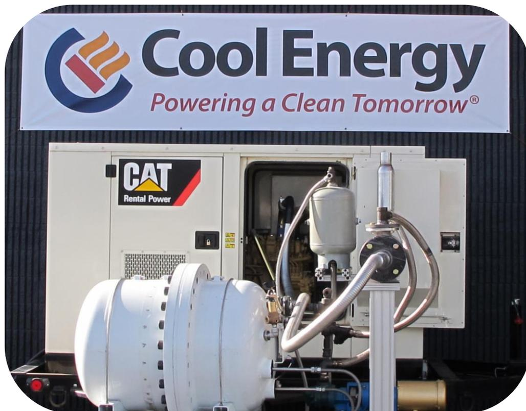
Fig 4) 3 kW<sub>e</sub> ThermoHeart® Engine boosting genset output by up to 7%.
