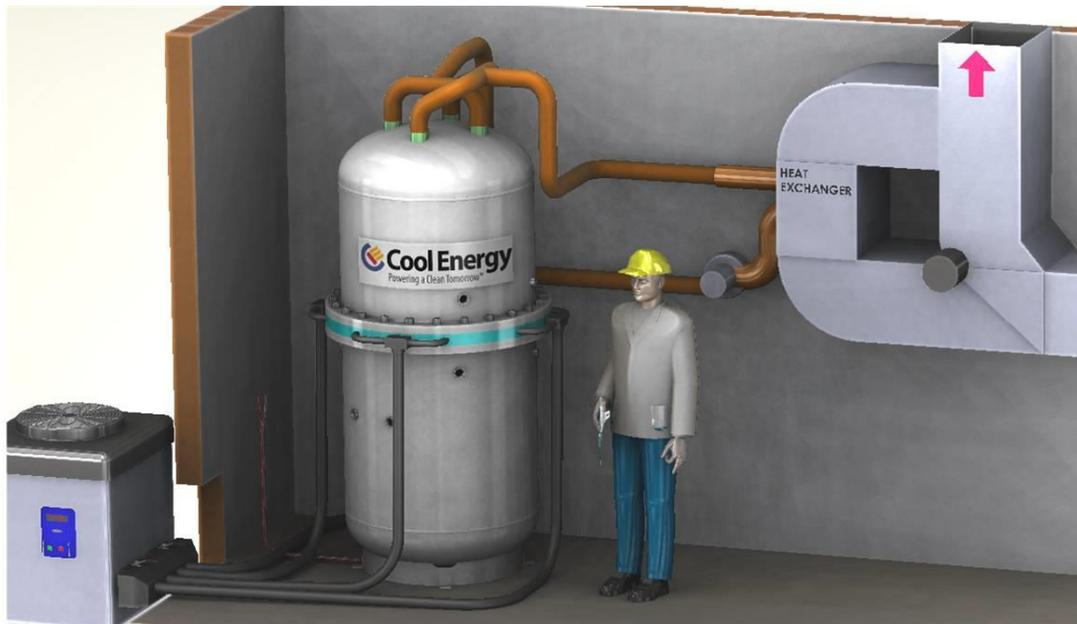
*Figure 2) Rotary-drive 25 kW<sub>e</sub> Stirling engine shown in an example waste heat recovery application. The source of hot gas flowing through the engine heat exchanger could be a reciprocating engine exhaust stream, or waste from an industrial process or pollution control equipment. Gas temperatures up to 600°C can be used, even though the heat transfer fluid used to deliver thermal energy to the engine will not exceed 400°C.*
