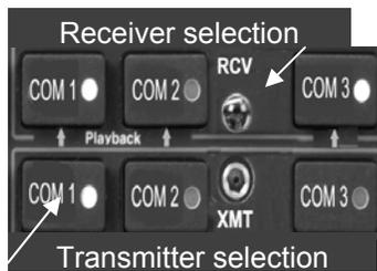
To select COM 1 COM 2 or COM 3 for transmit, press the button on the bottom row, next to the XMT legend. The bottom and top button indicators light, showing that you will transmit **and** receive on the selected radio.
