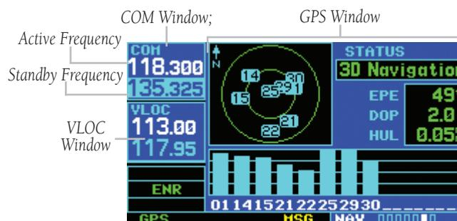
Each unique screen of information is referred to as a page. Pages are typically selected using the small and large right knobs, with the cursor removed from the GPS Window. See pages 6 and 7 for details on arrangement of the GNS 430's main pages.
