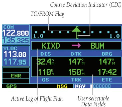
The following symbols are used on the Default NAV Page (directly below the CDI), to depict the 'active leg' of a flight plan or direct to:
