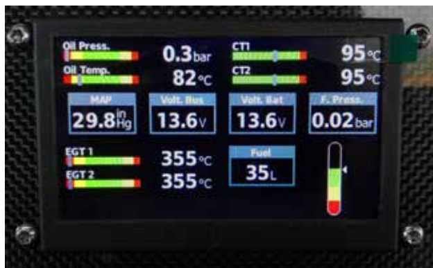
ALPHA Trainer Engine Management System display - example of data presentation
