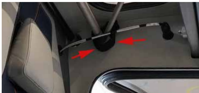
BPRS installation: belts attachment points to fuselage structure
